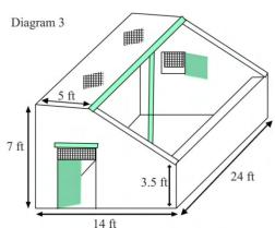
for a 5-ft wide roof. The slope should be away from the homestead (if the shed is attached to the home), to avoid accumulation of snow and rain. The main beam of the roof will be supported either by a central pole with an extra 6-ft beam or by a partition wall, but that would take up more space. In addition to the roof openings, as demonstrated in diagram 2, windows should be provided to facilitate air circulation (see diagram 3). All openings should be covered with wire mesh. To
